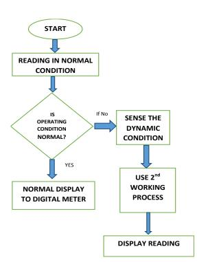
Fig4: Flow chart of the working of the meter
