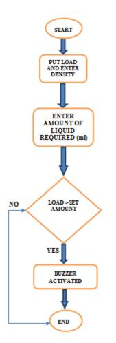
Fig5: Flow Chart of the working of meter
